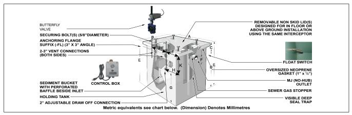
Note: The "C" dimension detailed above is from either the middle of the inlet or the outlet to the top the interceptor. The inlet and outlet dimensions are always the same.
