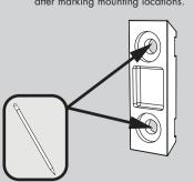
If mounting directly to wood stud, Plastic Anchors are not required. If mounting to tile, acquire proper mounting hardware capable of supporting the accessory in use. If mounting to drywall, drill guide holes at marked locations using a Drill equipped with a Ø 3/16" bit.
