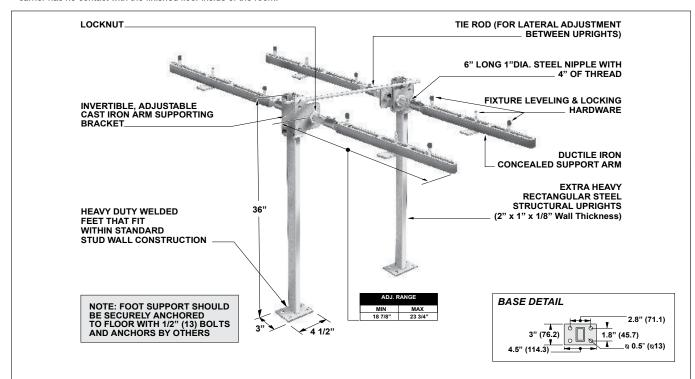
MC-42D Series Meets ANSI/ASME fixture carrier standard A112.6.1M-97
