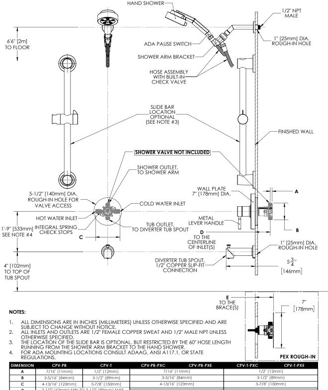
2-1/2" (63mm) MIN TO 3-1/2" (89mm) MAX D 3-3/16" (81mm) MIN TO 4-3/16" (106mm) MAX 3-1/8" (79mm) MIN TO 4-1/8" (105mm) MAX Ε
