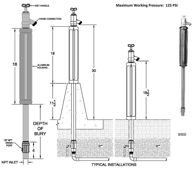
For Vehicular Traffic Areas Concrete Bollard May Be Desirable
