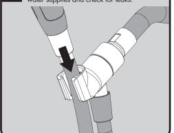
Ensure Hose Washer is inserted inside connector to avoid leaks. Thread Hose End with Label to base of Hand Shower. Hand tighten. Remove label.
