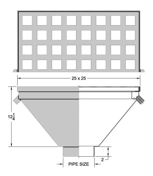
**Regularly Furnished:** A.R.C. steel flushing rim floor sink with deep sump body, anti-tilt loose set grate, & two 1/2" flushing connections. Grate openings: 2" Square.
