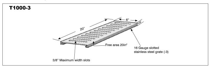
**Specification:** MIFAB® Series T1000-F-3, 6" wide x 20" long stainless steel trench drain grate and frame. Grates to have maximum 3/8" openings. Supply in sections as indicated on drawings.
