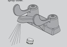
Shut off water supplies. Remove old faucet. Place faucet through mounting holes in sink. Secure faucet to sink using mounting nuts (1) provided.
