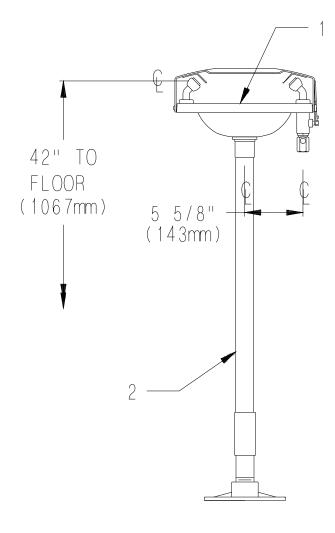
NOTE: This unit should be connected to an uninterrupted source of potable water, with a minimum flowing pressure of 20 PSI and a maximum static pressure of 125 PSI.
