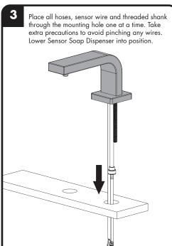
From beneath, reinstall the Rubber Washer (1), Metal Washer (2) and Mounting Nut (3) to secure the Sensor Soap Dispenser. Align the Sensor Soap Dispenser to desired position and wrench tighten Mounting Nut (3). Verify that the wires are not pinched.
