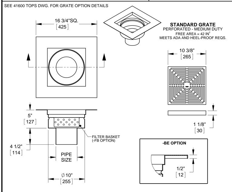
OUTLET O.D. FITS CLOSELY WITH I.D. OF NO-HUB CAST IRON PIPE
