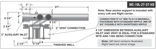
**Note:** 14 1/2" (368) minimum space required between front of foot supports. 9" (229) minimum in wall space required between back of in wall foot supports. **Note:** Foot supports and faceplate are assembled at the factory before shipment in the typical siphon jet water closet configuration and are reversible for the blowout water closet design.
