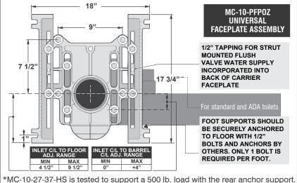
\*MC-10-27-37-HS Series Meets ANSI/ASME fixture carrier standard A112.6.1M-97 500Lb. Load Rating
