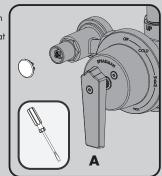
B. Secure the included "Key" to the Stop Valve using the included Screw and turn clockwise to shut "OFF". Repeat for Cold Supply Stop Valve.
