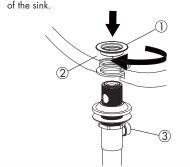
Make connections to water lines. Use 1/2" IPS faucet connections (1), or use 3/8" O.D. ball nose risers (2) with coupling nuts (3). Use wrenches to tighten connections. Take care to not overtighten.
