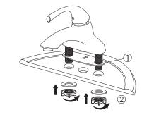
Place the rubber washer (2) to underside of the flange (1). Insert the threaded end of the drain body up through the drain hole and attach flange to the body with the pivot hole (3) pointing to the rear of the sink.
