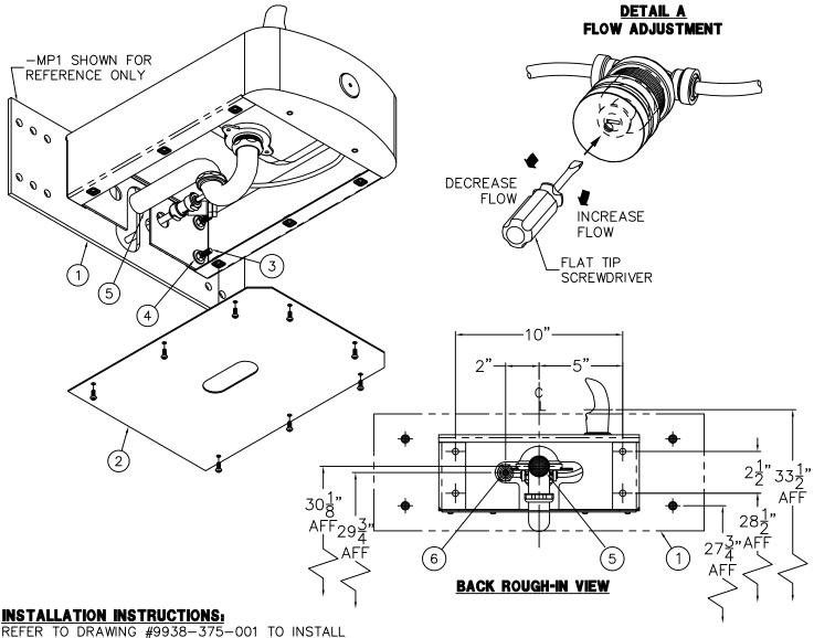
REFER TO DRAWING #9938-375-001 TO INSTALL -MP1 WALL MOUNTING PLATE.
